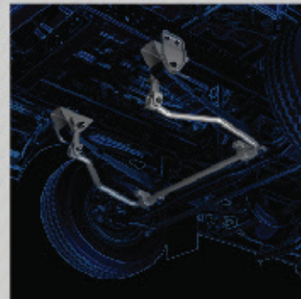
Front and rear parabolic suspension with anti-roll bar for better control and balance
