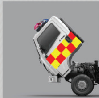
Tiltable cabin for better serviceability
